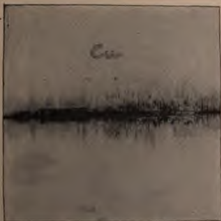
DEFLAGRATED COPPER WIRE.
